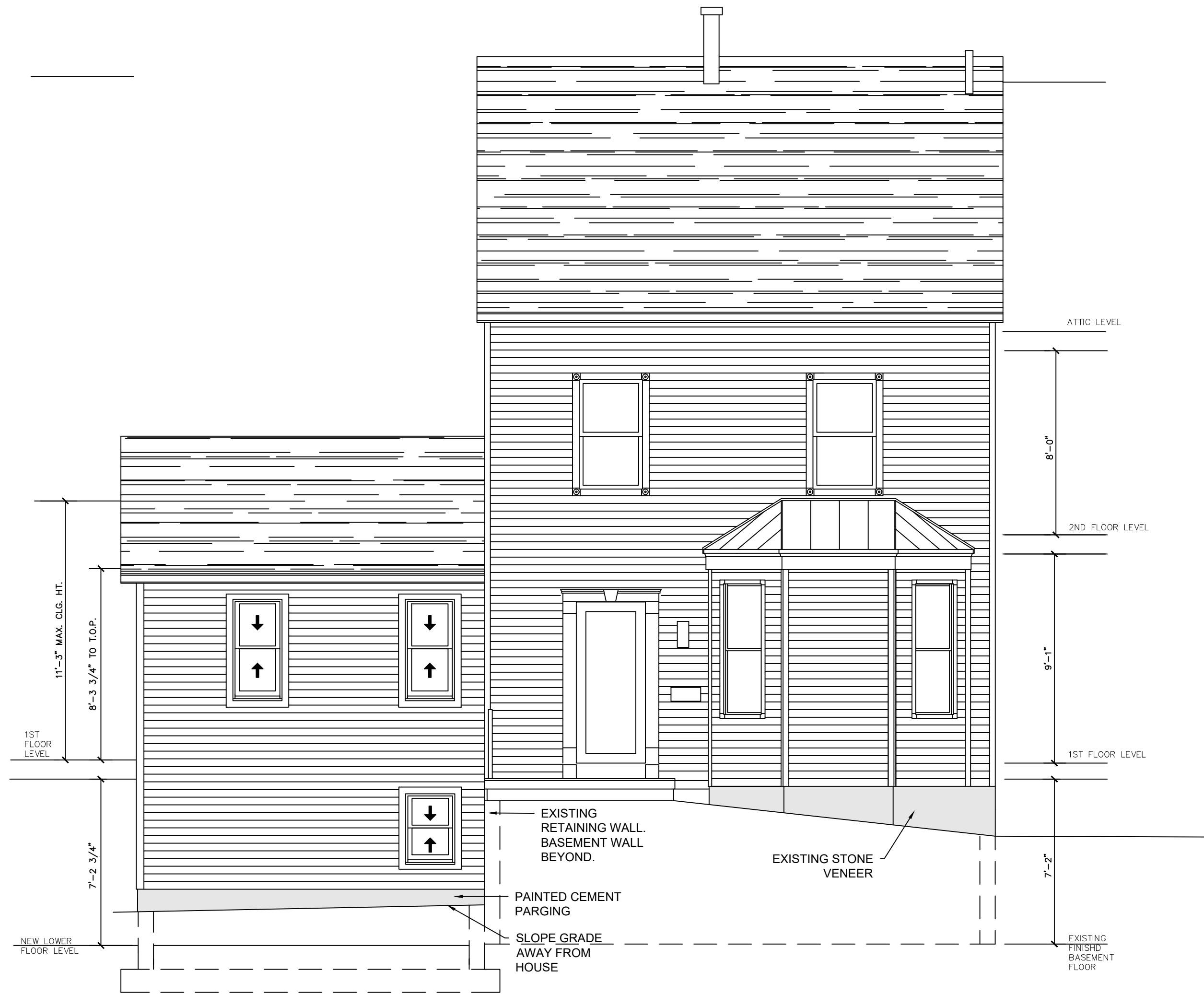
1 A-3 PROPOSED FRONT ELEVATION ( WEST ) SCALE: 1/4" = 1'-0"
