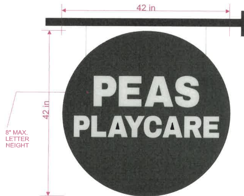
6MM DOUBLE SIDED ALUMINUM SIGN - DIRECT U.V. PRINTED
