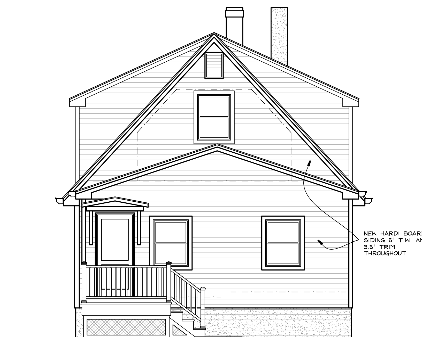
1 NORTH (FRONT) ELEVATION A2 1/4" = 1 FOOT
