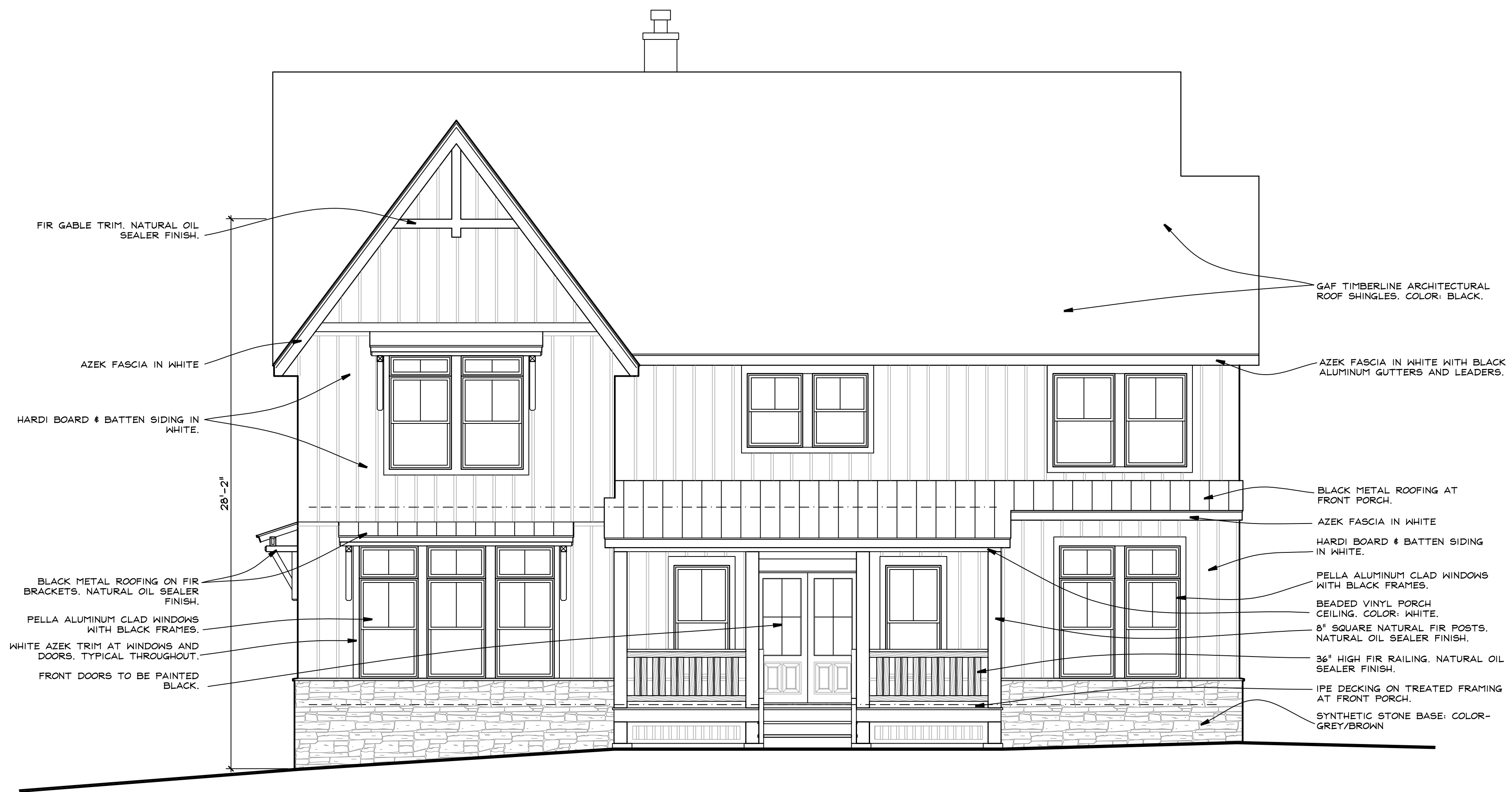
(A) FRONT (NORTH) ELEVATION A4 1/4" = 1 FOOT
