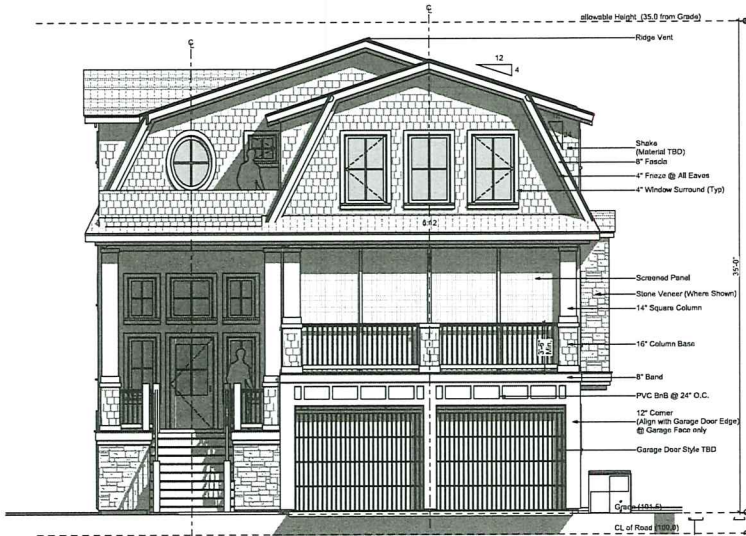
2 A201 North Elevation SCALE: 1/4" = 1'-0"
