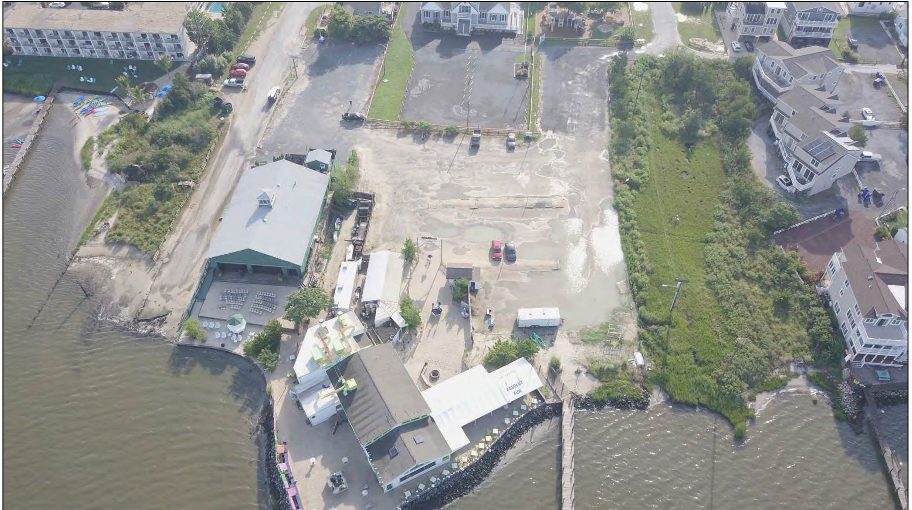
Figure 4. Drone image of the proposed project area. Note that the end of Dagsworthy St. (left) has fallen into Rehoboth Bay due to erosion and shoreline loss. Note also the sediment left on roads and parking areas by flooding. Approximately two feet of shoreline loss per year is occurring.
