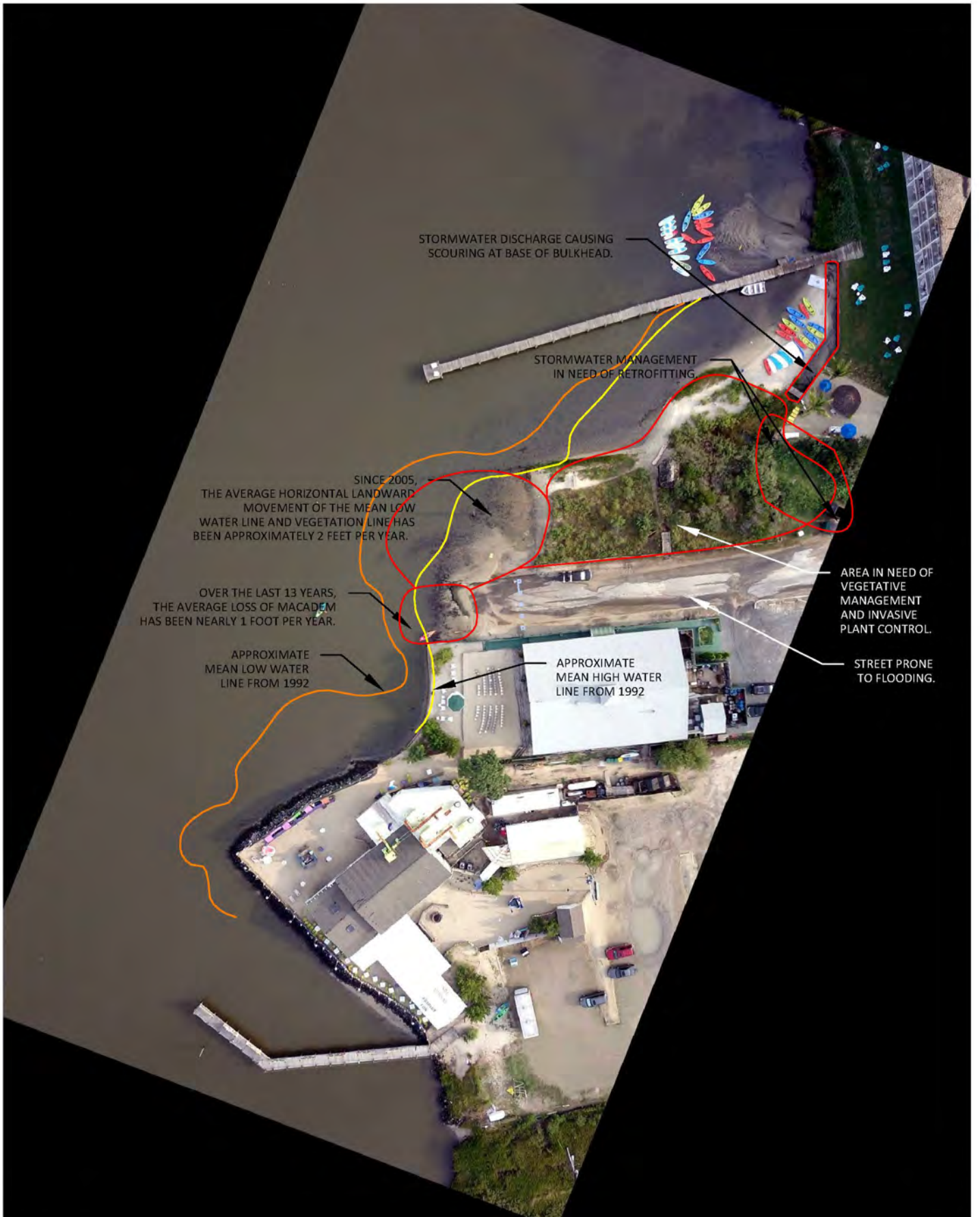
Map showing issues to be addressed by the proposed project. These include: average loss of 2 ft/yr of shoreline and beach since 2005; average loss of roadway macadam of 1ft/yr; chronic flooding of Dagsworthy St.; aging stormwater infrastructure; and invasive vegetation in Sunset Park.
