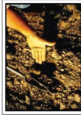
Fig. 5. Augered from a depth of 19 inches below the surface of the replaced topsoil, this subsoil sample was hand rolled to a 1/8-inch diameter. The test shows the soil at this site stretches out too far without crumbling; it indicates the material is in a plastic state of consistency, too wet for final decompaction (deep subsoiling) at this time.
