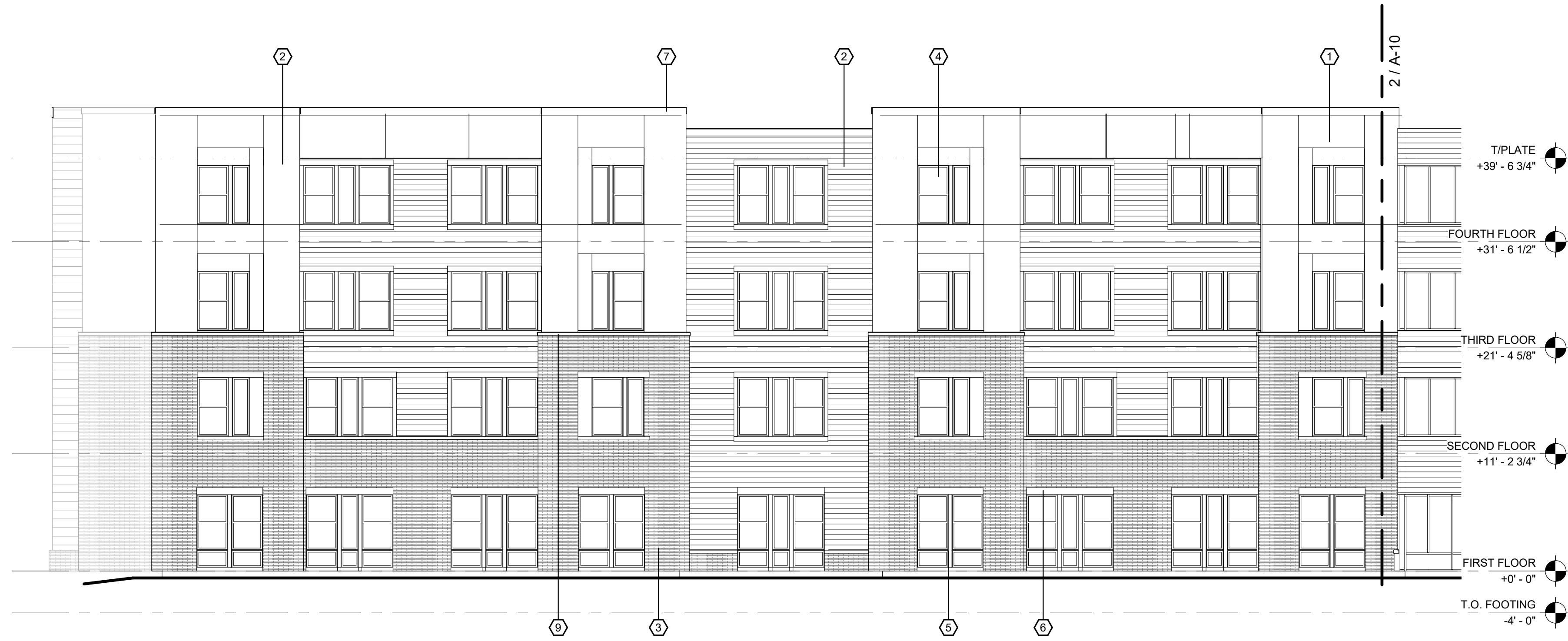
3 EXTERIOR ELEVATION - EAST 1/8" = 1'-0"
