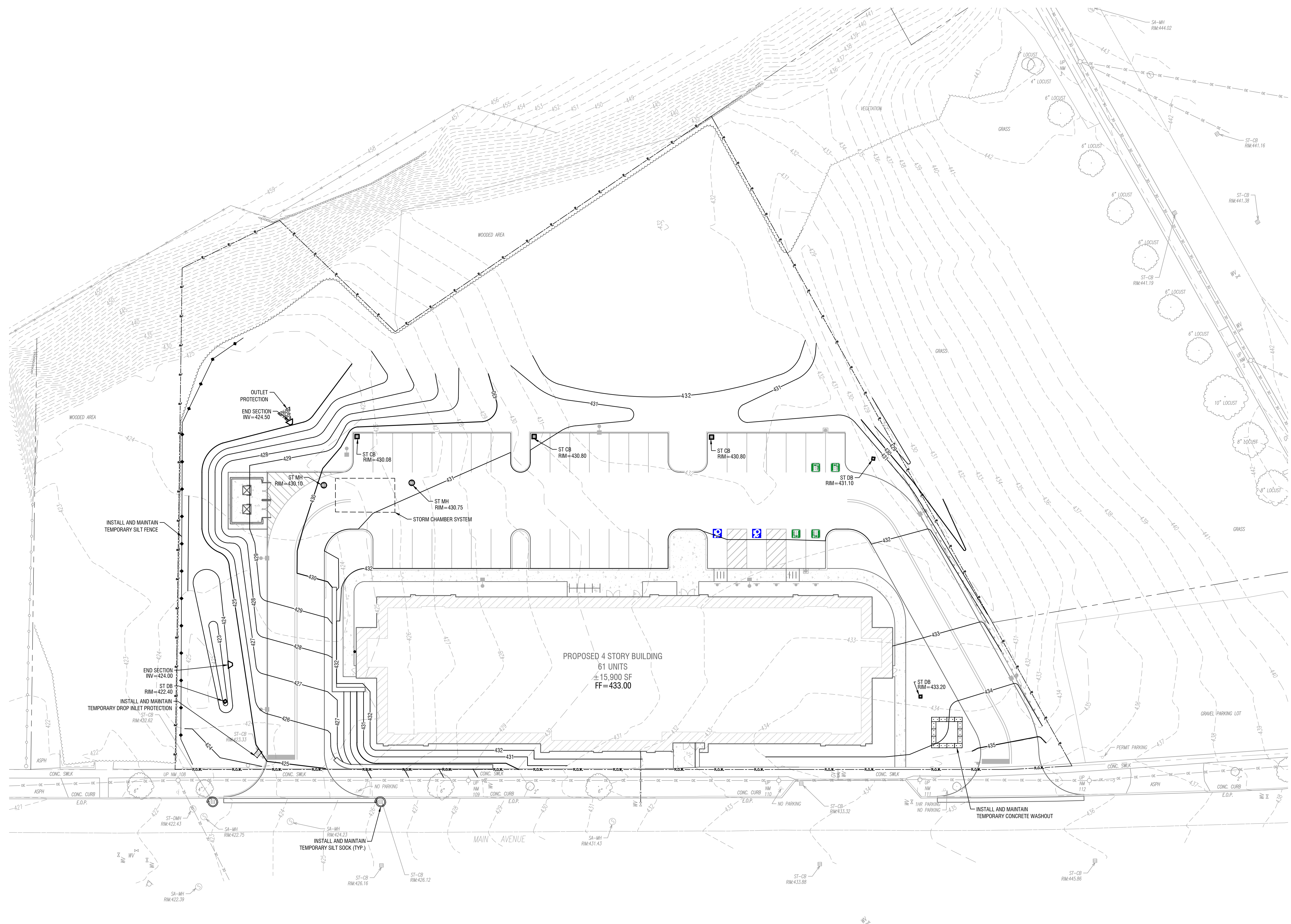
1 GRADING AND EROSION CONTROL PLAN SCALE: 1" = 20'
