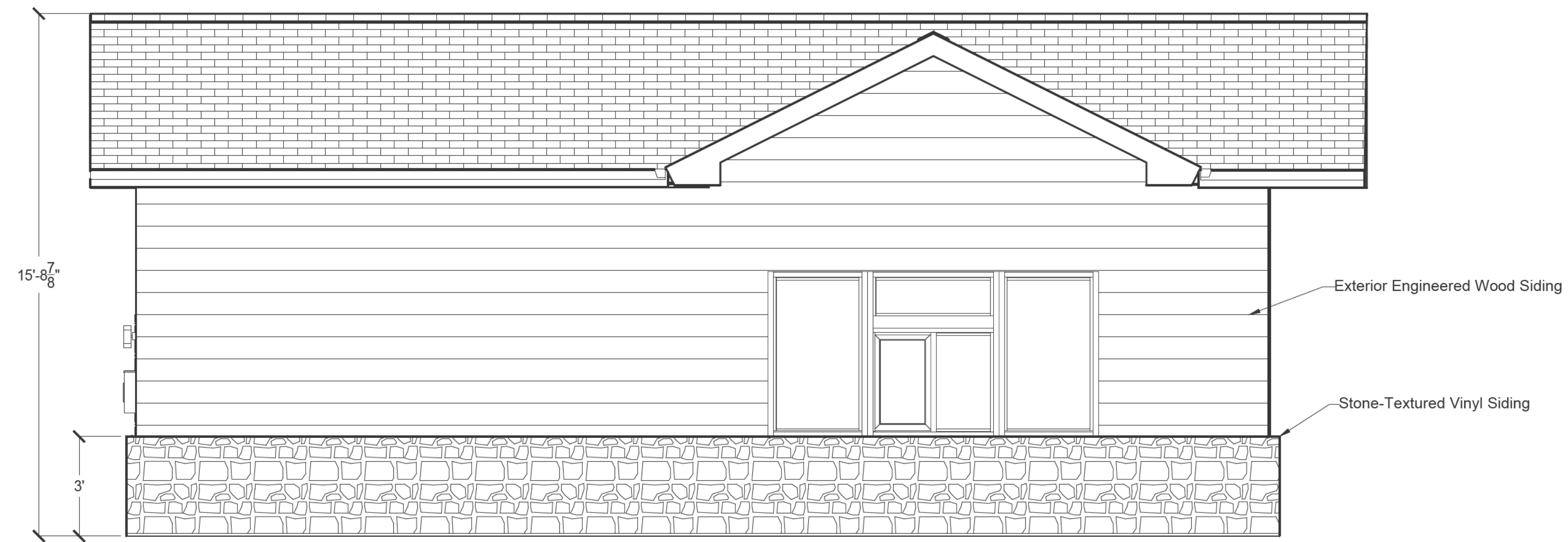
EAST ELEVATION (WEST ELEVATION SIMILAR) SCALE: 3/8" = 1'-0"
