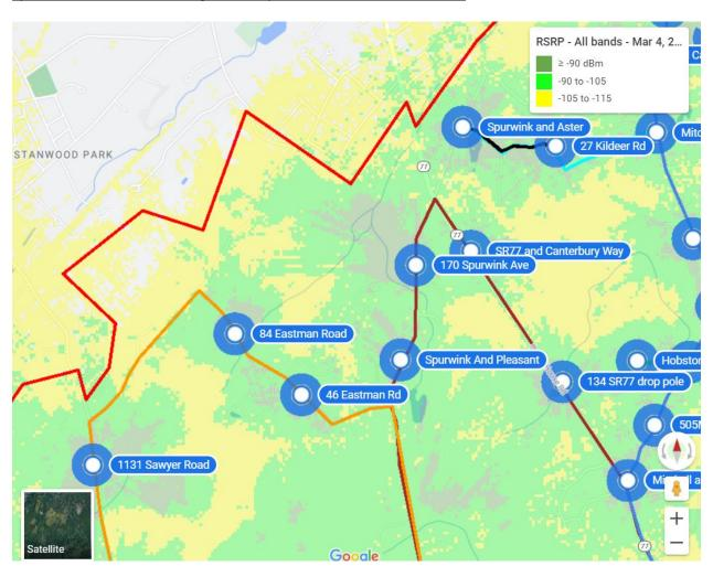
The colored lines show the proposed fiber optic cable routes to connect all these proposed sites. The blue loop is the western portion of the Mitchell Road and Shore Road loop. The dark brown loop in the middle is the northern portion of the main fiber loop, the orange loop on the left is the northern portion of the Sawyer/Spurwink Roads loop. The black and light blue lines at the top represent short fiber connections to proposed sites that aren't on the main fiber routes.
