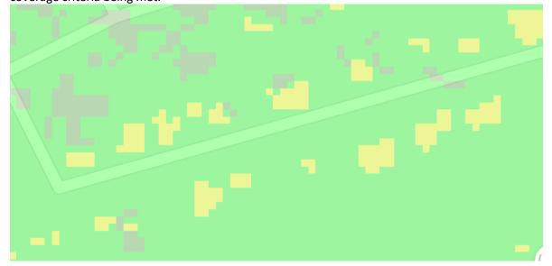
Below is an example of a portion of a building that might not have complete wireless coverage. It shows predicted coverage below -115 dBm RSRP at the northern portion of the building.
