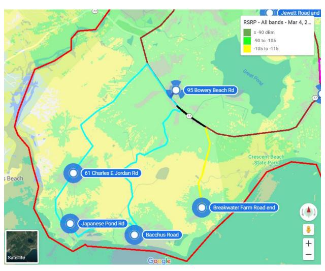
The colored lines show the proposed fiber optic cable routes to connect all these proposed sites. The dark brown loop in the upper right is the southern portion of the main fiber loop, the light blue loop on the left is the Monastery Road loop. The yellow line is to connect one site to the Main fiber loop. The red line is the town boundary for Cape Elizabeth.
