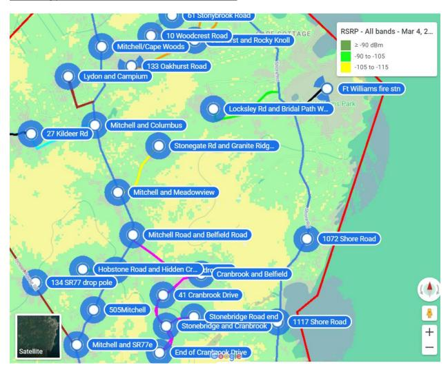
The colored lines show the proposed fiber optic cable routes to connect all these proposed sites. The blue loop is the middle portion of the Mitchell Road and Shore Road loop. The orange, violet, brown, yellow, black, green and light blue lines represent short fiber connections to proposed sites that aren't on the main fiber routes.
