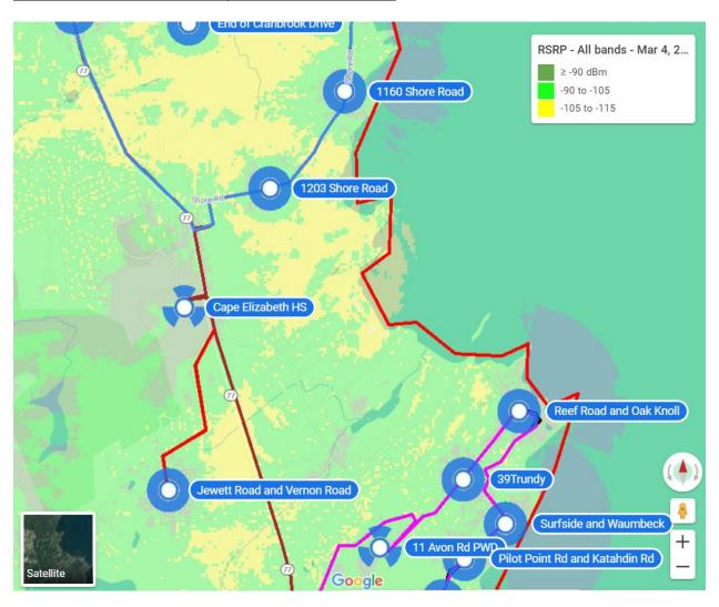
The colored lines show the proposed fiber optic cable routes to connect all these proposed sites. The blue loop at the top is the southern portion of the Mitchell Road and Shore Road loop. The dark brown loop in the middle is the eastern portion of the main fiber loop, the purple loop in the lower right is the northern portion of the Broad Cove loop. The red line on the lower left is a fiber connection along Fowler Road to connect one site that doesn't lie on any of the fiber loops.
