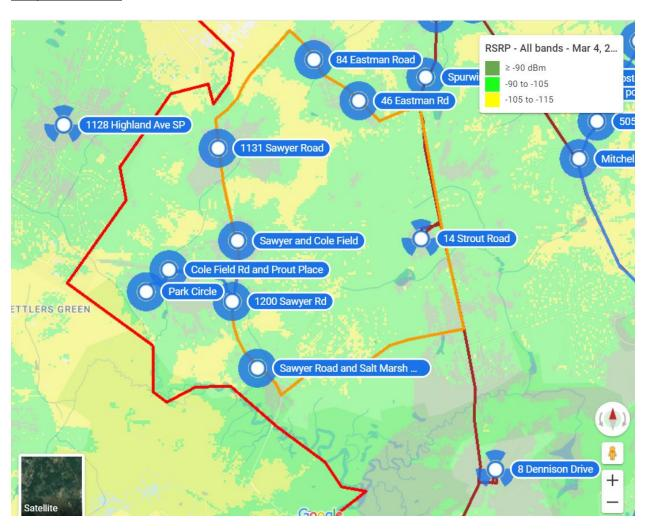
The colored lines show the proposed fiber optic cable routes to connect all these proposed sites. The blue loop on the right is the western portion of the Mitchell Road and Shore Road loop. The dark brown loop in the middle is the northwestern portion of the main fiber loop, the orange loop in the middle is the entire Sawyer/Spurwink Roads loop.
