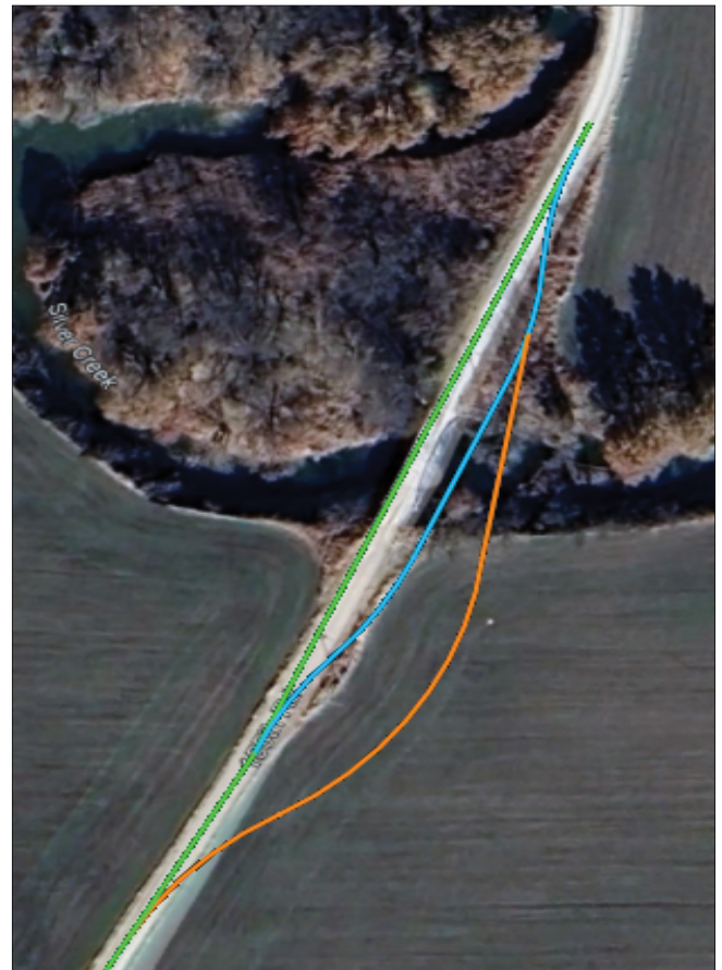
(3) Blue - Parallel to Existing Alignment 50' offset CL; Orange - Near Perpendicular to Channel (Approx., not final)
