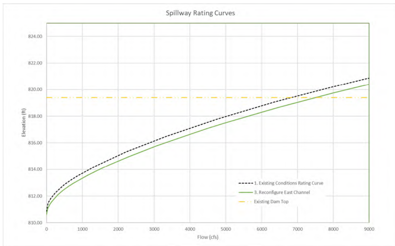
Figure 3.3-2 GeoHECRAS Rating Curve – Reconfigured East Channel Compared to Existing Conditions
