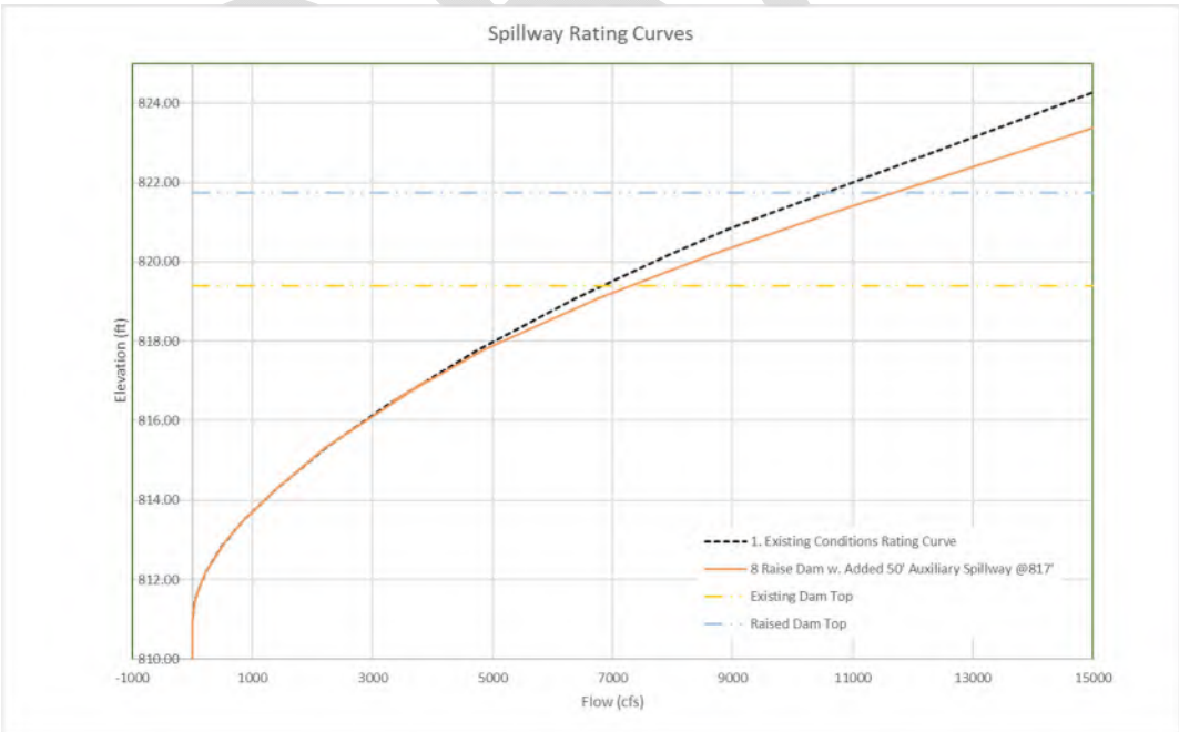
Figure 3.8-2 GeoHECRAS & Weir Equation Rating Curve –Raised Dam and Added Auxiliary Spillway Compared to Existing Conditions
